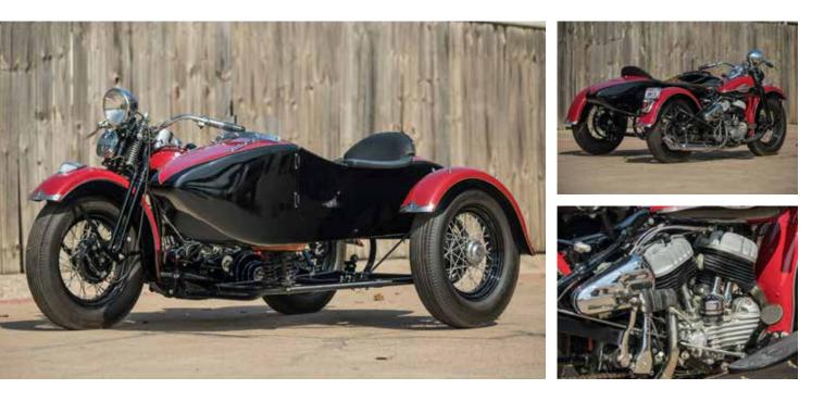
In 1937, Harley Davidson introduced a new series model called W that featured a 45 cubic inch engine and more importantly a recirculating oil system that was supposed to reduce maintenance and increase reliability. This was specifically convenient for the rider that did not need to check the oil, adjust the oil pump or even lubricate the engine while riding anymore. Harley quickly received an order from the US Army to replace its fleet of RL models.
