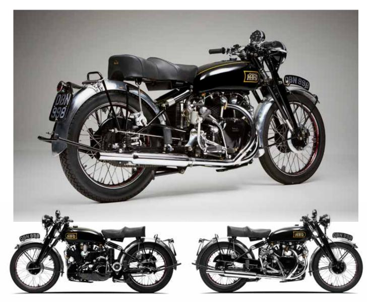
The most significant changes made concerned the suspension, there being a revised arrangement at the rear incorporating curved lugs for the seat stays and an hydraulic damper between the spring boxes, while at the front the new models boasted Vincent's own 'Girdraulic' fork: a blade-type girder fitted with twin hydraulic dampers.
