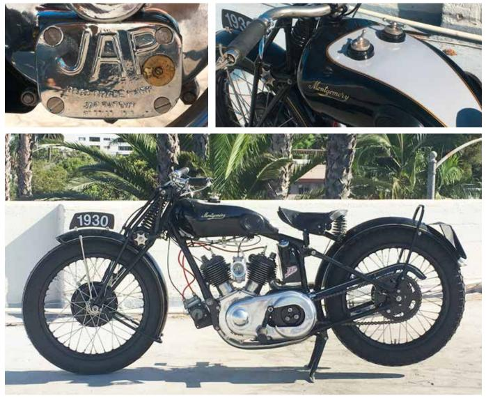
This J.A.P. engine is a sidevalve motor of 750cc displacement with air-cooled covers over the exhaust valves. The highly polished engine cases are a delight to enjoy. Ignition is provided by magneto located forward of the engine. An Albion gearbox with a 3-speed hand shift completes the package. It can be described as a touring motorcycle capable of extended use at a high rate of speed. Unfortunately, World War II forced the small English company to shut down and production ceased in 1939.
